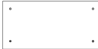
2. Panel Mechanically fixed to smooth wall or panel (concrete, plasterboard, timber panel, timber door or metal sheet)
